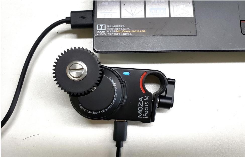
2. Connect iFocus M to the Computer using a USB type-C cable.
