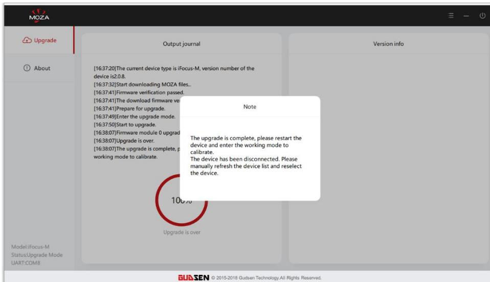
Note: The iFocus M will automatically calibrate after firmware upgrade. Calibration will take 10 seconds, a blue light will flash during calibration. When calibration is finished disconnect the iFocus M from the computer. iFocus M is now updated and ready to be used with a MOZA gimbal.
