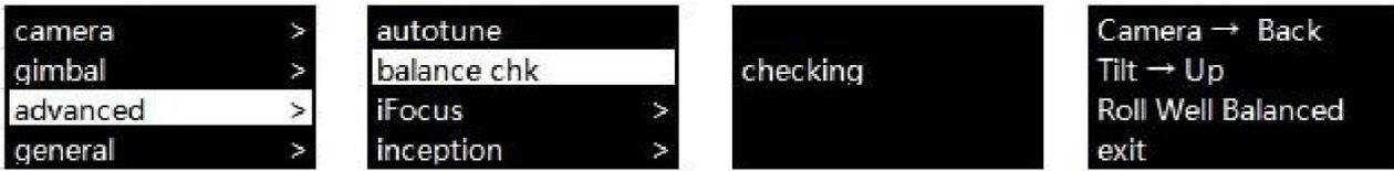
How to Access: Enter the menu, select advance>balance chk, and the gimbal’s system will start to check the balance of each axis.
