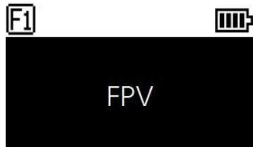
How to Access: Triple press the Fn button to enter the FPV Mode. Triple press again to exit the FPV Mode.
