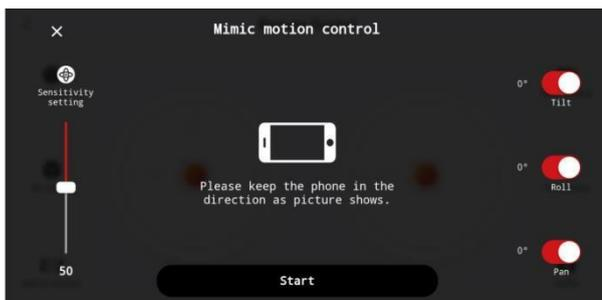
How to Use Mimic Motion Control: Through the MOZA Master app enter mimic motion control, click the 'Start' button, then rotate the phone. The gimbal will mimic the direction and speed of the phone's movement. The sensitivity of mimic motion control can be adjusted on the left. On the right, each axis's movement can be turned off or on.
