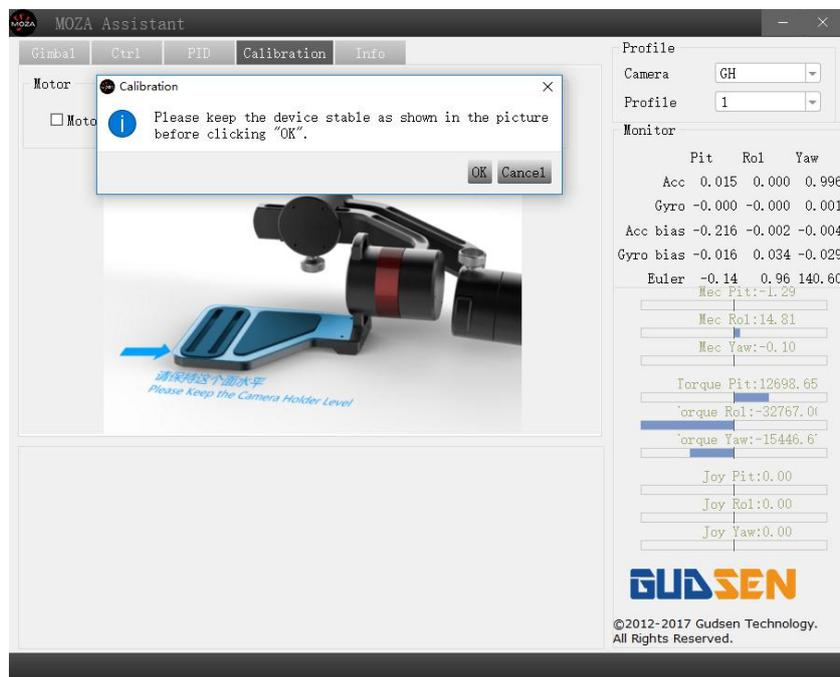
⑥ Please make sure the Camera Holder is horizontal against the surface of the desk, then click on the "OK" button to begin the calibration, Software interface will show on when it is a successful calibration ( It takes about 5-10 seconds to do the accelerometer calibration).
