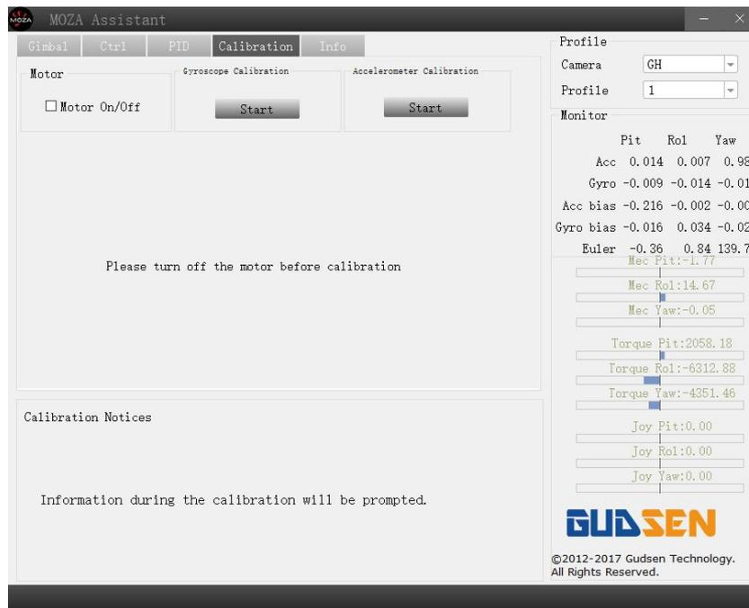
④ Click on "Start" button under gyroscope calibration, Software interface will show on when it is a successful calibration ( It takes about 5-10 seconds to do the gyroscope calibration).
