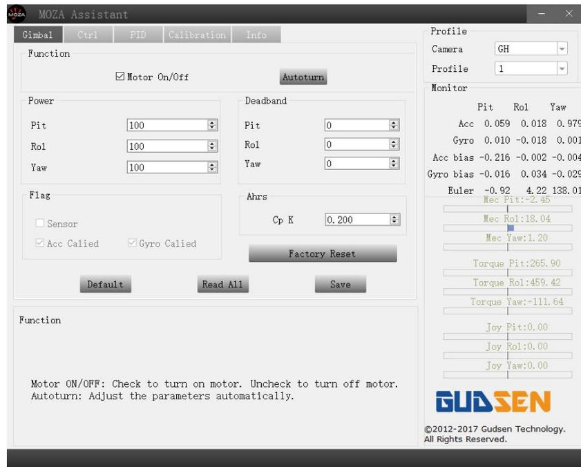
②Uncheck the "Motor On/Off" on the calibration interface.
