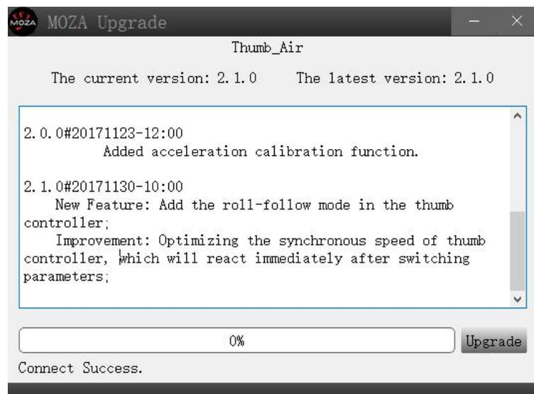
②Ensure the network being connected, MOZA-Assistant will display information of firmware version and upgrade, click "Upgrade" to start upgrading the thumb controller. When the update is done, the thumb controller display will show the "Upgraded OK" information, the firmware update for wireless thumb controller is completed!
