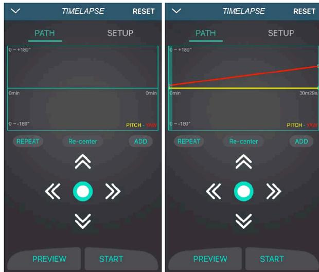
Tap setup to set 'Shutter Interval', 'Shutter Duration'(shorter than 'Shutter Interval'),'Target Clip FPS 'and ' Target Clip Length'.
