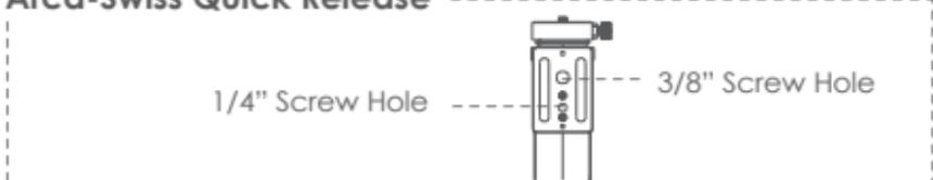
There is a 1/4" screw hole and a 3/8" screw hole on the body of Arca-Swiss quick release which can meet various extension needs. (When connecting the body with monopod or tripod via the Arca-Swiss quick release, the Slypod E can be used as a motorized slider)
