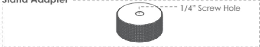
There are 1/4" extension screw holes on the stand adapter which enable the body to connect with tripod or other accessories to mount different shooting devices.
