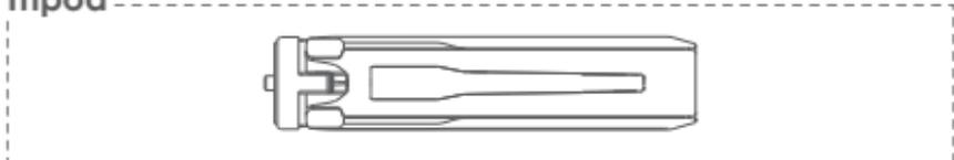
There is a 1/4" extension screw on top of the tripod, which can be used for support and extension, the tripod can be used as a handle when the legs are not open. (The main body must be connected to the stand adapter to connect the tripod)
