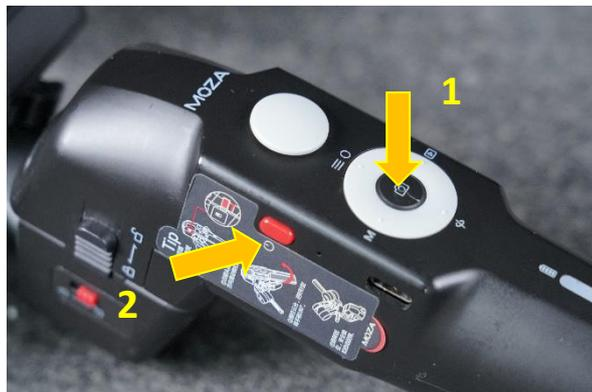
**power button.** The Led light will be flashing in blue-green-orange. Now the gimbal is in boot mode.
