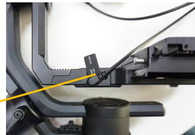
Fig2. Connect to the multi-can connector on Air 2 Gimbal
