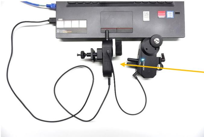
Fig5. Connect wireless handunit, ifocus motor and PC together
