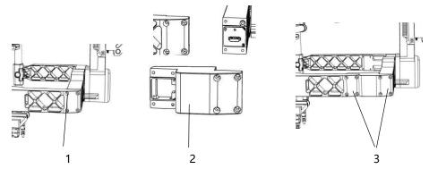
Take out 4 screws at [1], dismantle the rolling arm, and take out the roll-axis extension arm [1]. Fit the roll-axis extension arm to the parting position and use 7 screws to fix the port [3] to finish the installation.
