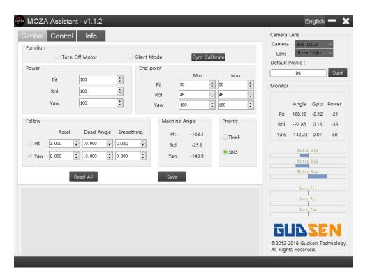
Turn off motor: Tick this box to shut down the motor's power. It's required to check this box before calibrating the sensor. Otherwise, data errors in the calibration may occur. Adjust the motor's working state and not make any noise. Check this box when audio is required.
