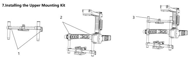
Loosen the tilt arm by loosening the knob at [1]. Insert the upper tilt arm to the connector [2] and tighten the knob.
