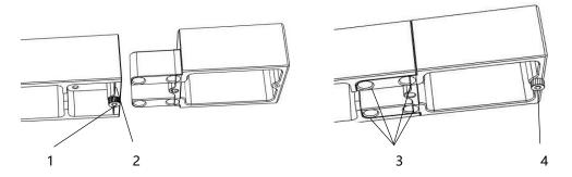
Loosen the screw [1], take out the baffle plate [2], and insert the extension arm into the yaw axis. Secure it with with 4 M4\* screws. Tighten it [4] with 1 M3\*10 cylinder head screw. You are now finished installing the yaw-axis extension arm.
