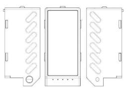
Each blue light indicates 20% power. The battery is charged when the last small light is blinking. The charge port is on the right.
