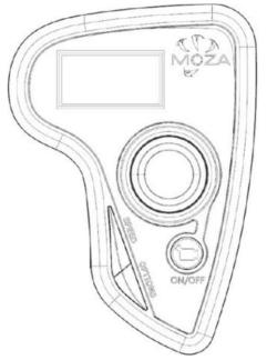
When charging the thumb controller in its power-off state, the screen will show "Charging" and indicate the battery level.
