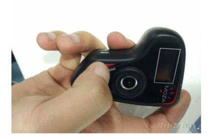
2 Plug in the USB cable, the "connecting" message shows on the OLED screen
