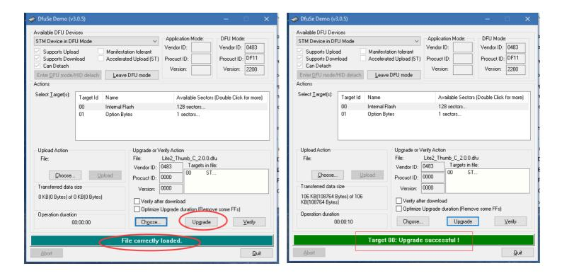
6. After the upgrade is completed, plug out the USB cable, restart the thumb controller.
