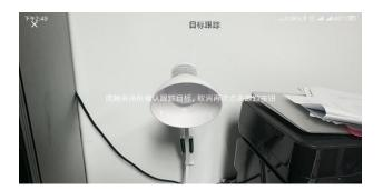
The object tracking function requires a smartphone to be mounted above the camera and running the MOZA Master App. (Phone
