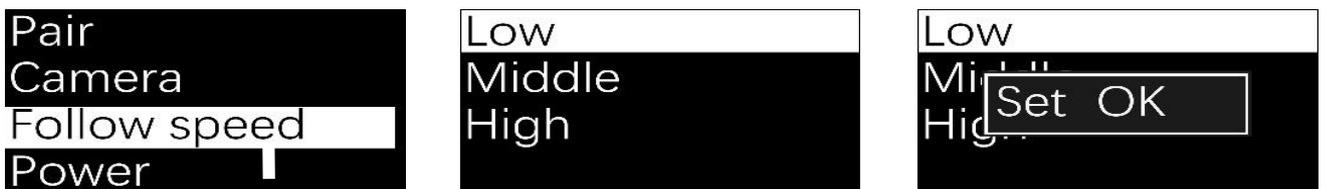
The specific figures of the different levels can be subtly adjusted with the MOZA Assistant software. After the adjustment, the thumb controller will display 'Set OK'. Otherwise it will display 'Set ERR'. In this case, it must be reset.
