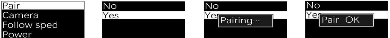
Every MOZA gimbal is properly paired before shipping. There is no need to pair again. Pairing failures may happen when the thumb controller firmware does not match the gimbal firmware. You have to upgrade both the wireless thumb controller and gimbal firmware to the latest version.
