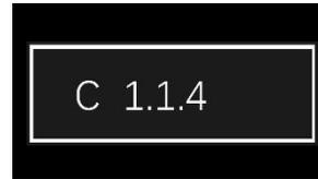
The front data is the hardware's version and the back data is the firmware version.
