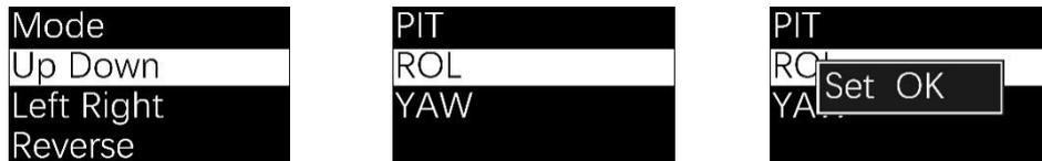
'Reverse' will make the power motor move the opposite way of the joystick. You can adjust according to your own needs. Operation direction has no relationship to the joystick map or the 4/8 Direction mode.
