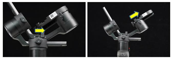
3. As shown in the figures below, loosen Roll knob, raise Roll arm to keep it out of groove of Pan motor crash pad, push down Pan motor lock and then you are ready to film now.
