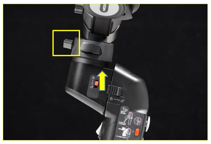
4. As shown in the figures below, loosen slide lock, rotate gimbal 180° along the direction of slide lock, then it locks automatically
