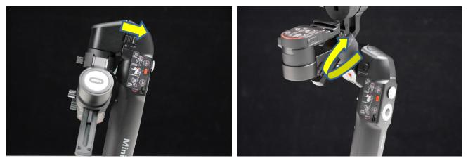
2. As shown in the figures below, push ejector pad on Roll arm to unlocked position, move Tilt arm upwards and then fasten Tilt knob.
