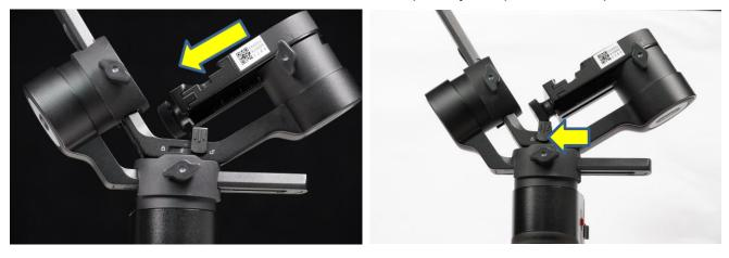
3. As shown in the figure below, rotate Pan arm, place Pan knob at outer side and push up Pan
