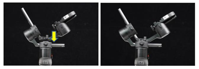
2. Push ejector pad on Roll arm to unlocked position first, as shown in the figures below, move Tilt arm backwards to end limit, fasten Tilt knob and then push ejector pad to locked position.
